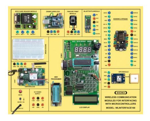
This trainer has been designed with a view to provide practical and experimental knowledge of Sensors programing with 8051 Microprocessor Board.
